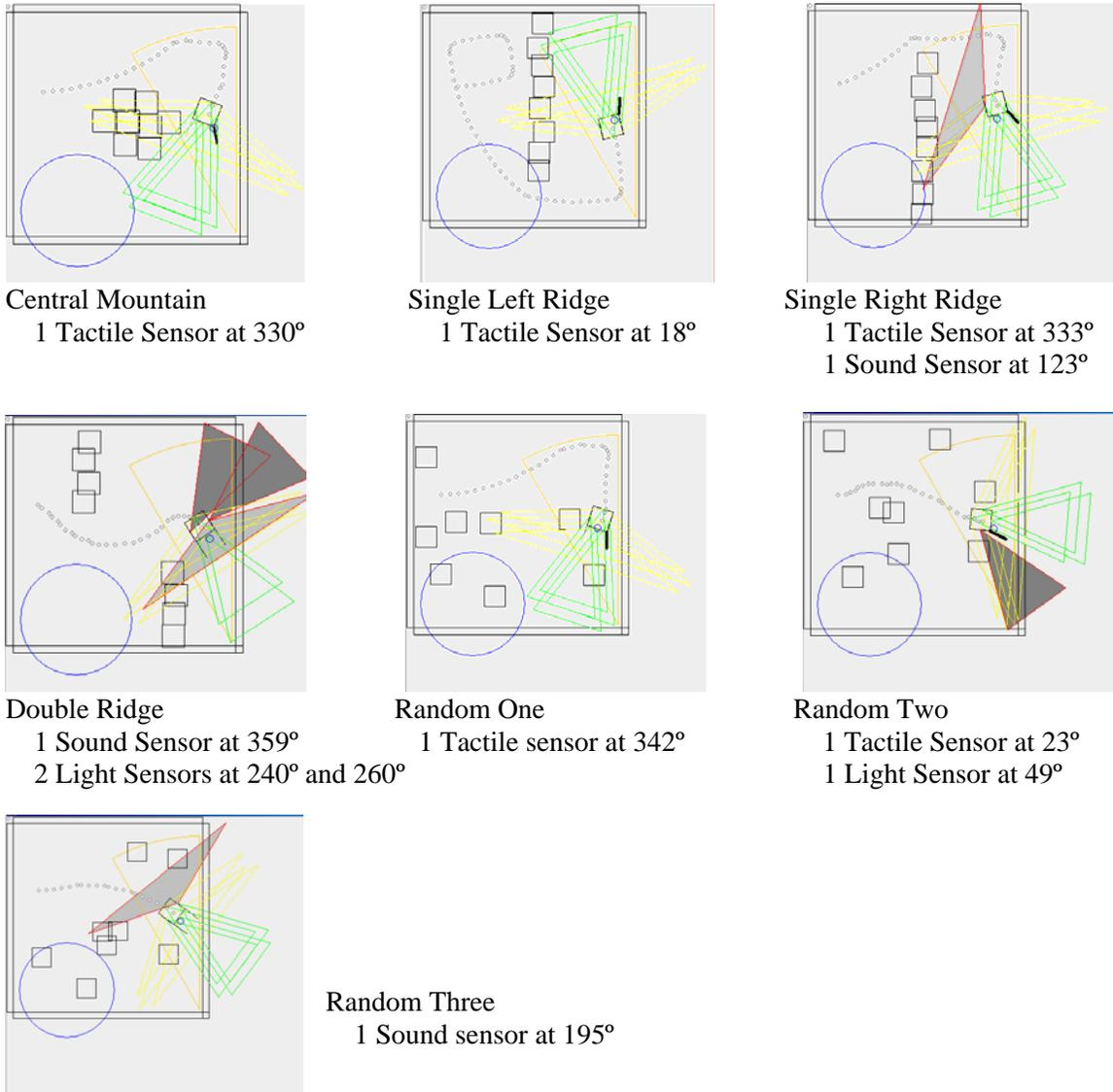
*Figure 5: Paths taken by elites. The sensors that were used are shown (darkened and filled in for ease of identification) along with the angle they were placed relative to the robot base. The unused sensors all point north relative to the robot base.*
