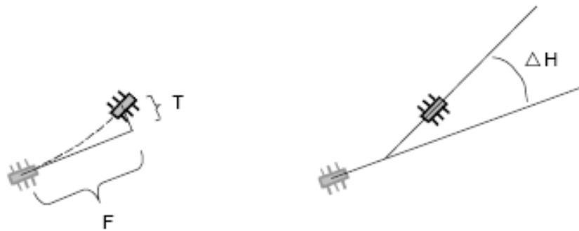
**Fig. 4** [19] Gait Cycle Turn Measurements: the diagram explains the turn gait of the robot. Given a start position, F is the distance moved forward, T is the lateral displacement and  $\Delta H$  is the change of heading from before to after a single gait cycle.
